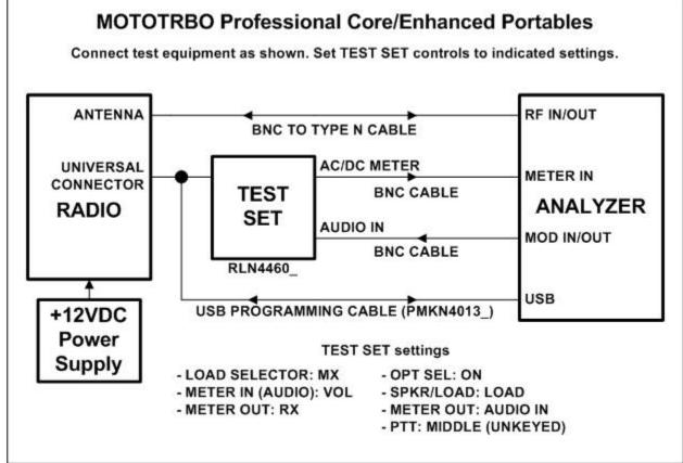
Figure 4-1. MOTOTRBO™ Portable Professional Core/Enhanced Test Setup Diagram
