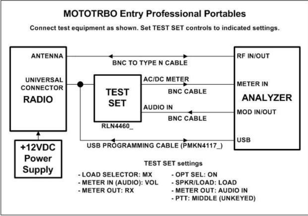
Figure 4-2. MOTOTRBO™ Portable Entry Professional Test Setup Diagram.
