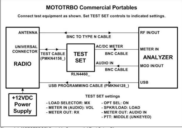
Figure 4-4. MOTOTRBO™ Portable Commercial Test Setup Diagram.
