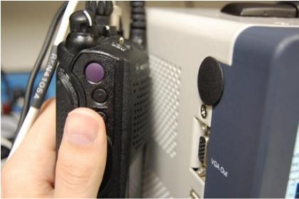
Figure 5-1. Place keyed radio next to analyzer speaker.
