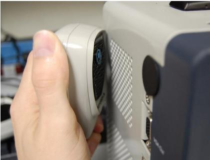
Figure 7-1. Place keyed radio next to analyzer speaker.
