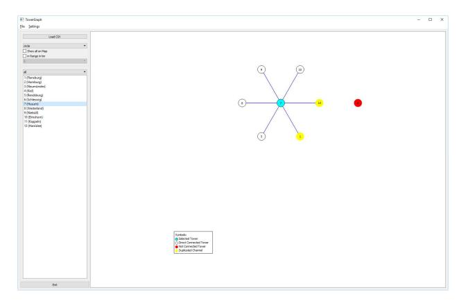
The circle graph provides a detailed comparison of the CURRENT with the DESIRED situation on the basis of measured data from the real-time operation, with display of the problems (for example, twice assigned frequencies in the object supply or in-correctly registered neighboring stations)
