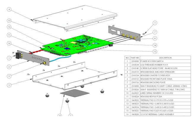
Figure 2: Embedded Chassis Assembly Deconstruction
