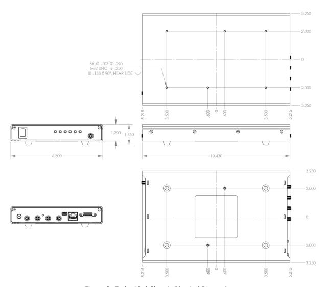
Figure 3: Embedded Chassis Physical Dimensions
